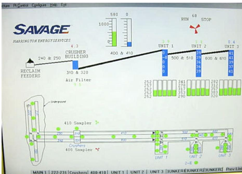
*fig. 8 - Harrington Station system status screen*
