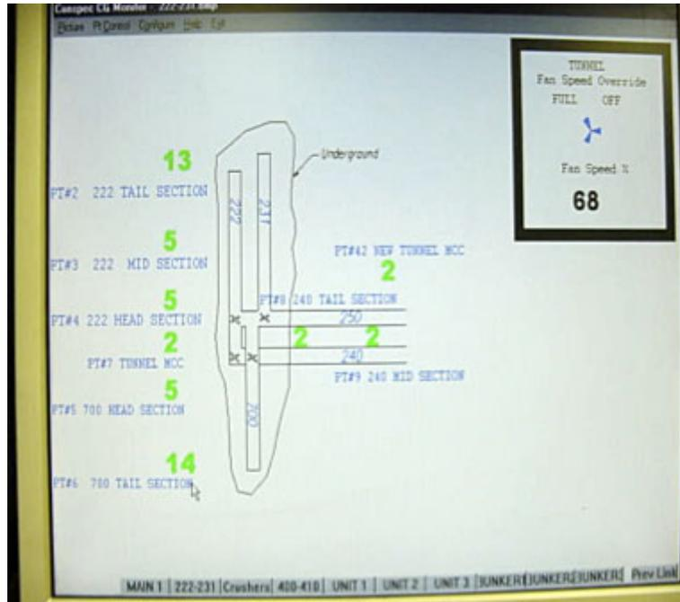
fig. 9 - Harrington reclaim tunnel CO concentration screen
