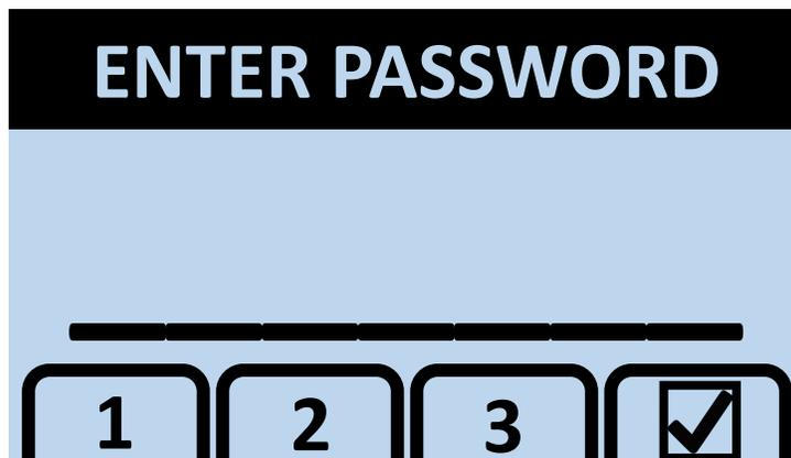
The default user password is "123". Once the password has been entered successfully, the user is taken to a screen to select which sensor will be calibrated. If the monitor is a single gas monitor, this step is skipped.
