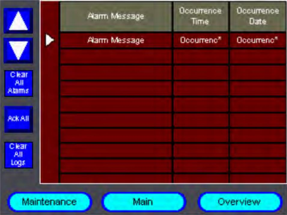
The Alarm Log screen logs alarms and error conditions. When an error occurs (such as a blocked probe during start up mode) the PLC immediately goes into alarm and energizes the trouble relay. This error is displayed on the panel view screen and needs to be cleared or acknowledged. A record of alarms and errors is kept in this screen and can be cleared if desired.
